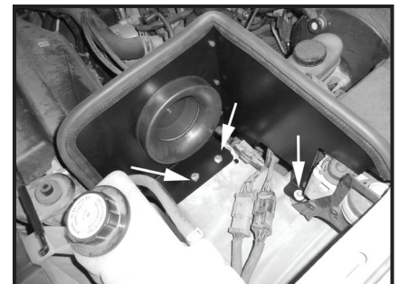
Step 15 Install the heat shield in location. Install the bolt and fender washer from the top side of the bracket. Install the lower mounting spacers and fasten securely in place with the supplied fender washer and nut. Install the bolt removed from Step 13.
